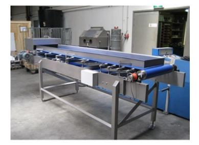
Standard Range or Customized Solutions Incorporate more control into your process than ever before with Rice Lake Weighing Systems' weigh belt feeders. Ideal for a wide variety of industries, including food, mining, quarries, bulk material blending, process control, truck, barge, or rail load-out applications, weigh belt feeders help ensure accurate and consistent weight output.
