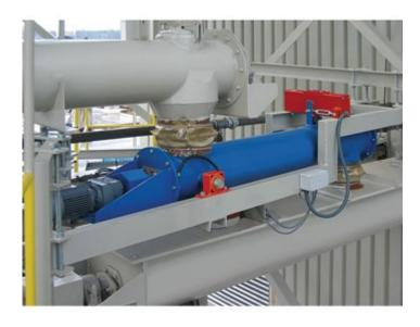
By providing an existing or new-to-build screw conveyor with a screw weigh system, one can easily create an in-line measurement without disturbing the product flow.
