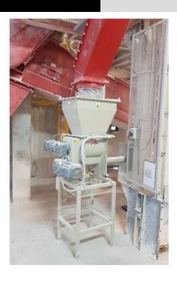
Loss-in-weight feeders are ideal dosing systems for a variety of applications from bulk, dry materials to liquids and even poorly flowing materials. Whether it's used in food or chemical production, high temperature or ATEX environments, Rice Lake Weighing Systems has a loss-in-weight feeder to meet your requirements
