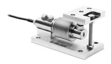
Mounting kit for FXC/FXD series bending beam <u>load cells</u> up to 500 kg, with single anti-tipping system and side force compensation. Fitted with ball joint for high-precision weighing.
