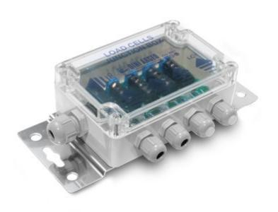
Simple junction box with IP67 protection and 4 inputs equipped with electronic board for junction of the signals of 2, 3 or 4 load cells. Screw terminal boards to facilitate the connection. The protection circuit protects against lightning and overvoltage. The reduced costs make it the ideal choice for static weighing systems such as silos, tanks and big containers.
