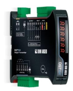
High-performance multifunctional weight transmitter, the fastest of the Dini Argeo range. It can manage up to 4800 readings per second, for weighing with precision in milliseconds. For DIN rail mounting, it allows direct reading and diagnostics of the connected weighing system. The wide range of available interfaces makes the integration of weighing into any automation system easier and safer.
