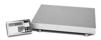
High precision floor balance for hazardous areas. Protection rating II 1G Ex ia II B T4 Ga for gas. CE-M approved (OIML R-76 / EN 45501).
