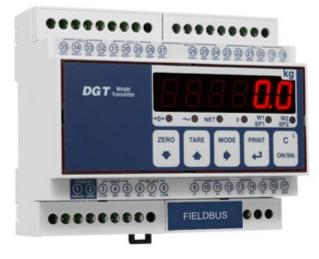
4-channel weight transmitter for weight transfer to PLC via fieldbus, analog output or RS485. It allows the reading and diagnostics of each load cell or each connected scale (up to 4).
