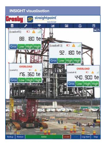
INSIGHT software, supplied with an SW-D USB wireless dongle, allows connection of up to 126 Straightpoint wireless load cells simultaneously onto any Windows tablet or laptop.
